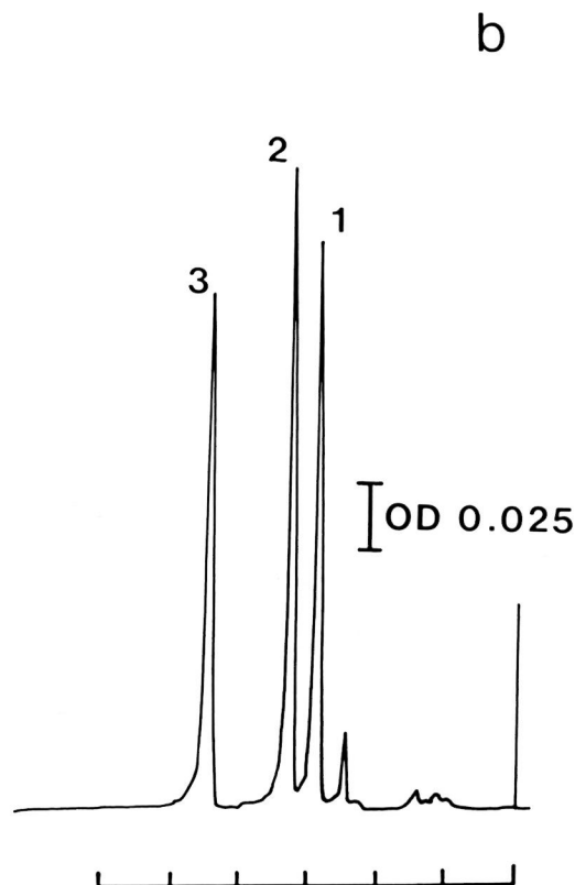
FIG. 2b. Reverse phase chromatogram of an extract of mouse plasma 2 hr after i.v. dosing with 50 mg/kg ETH plus TH. Peaks: 1 = TH, 2 = MTH (internal standard), 3 = ETH.
